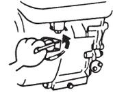
3. Turn the fuel valve to the "OFF" position.
